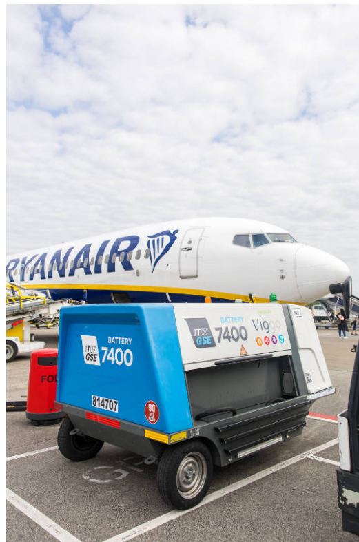
* Elektrische Ground Power Unit
